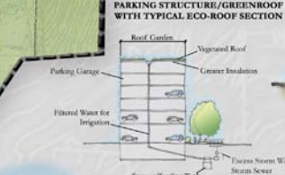
PARKING STRUCTURE/GREENROOF WITH TYPICAL ECO-ROOF SECTION
